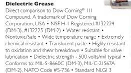
SILICONE COMPOUND DM is a premium silicone compound for use in a wide variety of applications. Its low volatility, non-melting thickener and high dielectric strength make it the compound of choice for moisture proofing ignition systems, spark plus connections, elect
